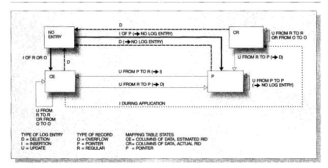
Figure 9 State transition diagram for an old RID's mapping table entry during processing of the log
